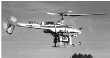
Figure 10.2. The CMU Yamaha R50 helicopter in autonomous flight.
