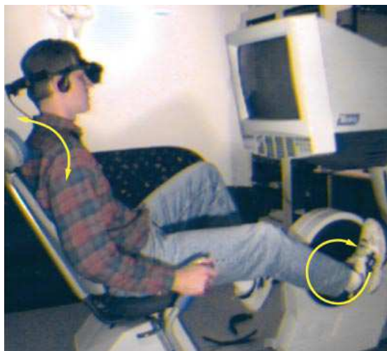
4 The Tectrix stationary bicycle that serves as the interface to the Border collie environment.
