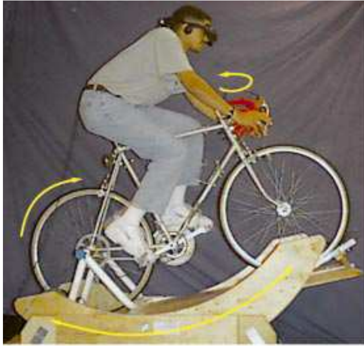
11 The user rides a racing bicycle mounted on a platform.
