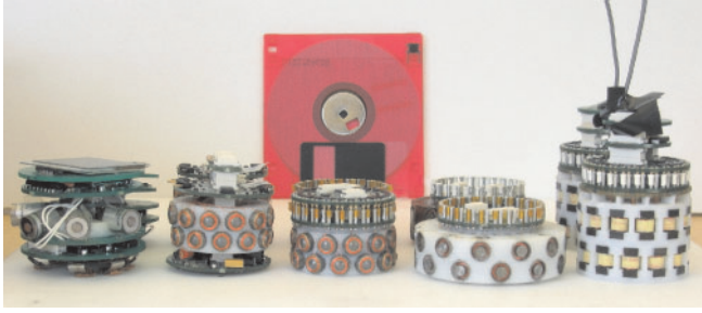
Fig. 16. Cylindrical, self-reconfiguring robot modules constructed in the Claytronics project which demonstrate rotational self-reconfiguration is possible. Each module is approximately 5 cm in diameter.
