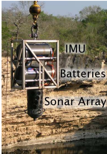
Figure 3: The Dropsonde as it is being lowered into Zacatón.
