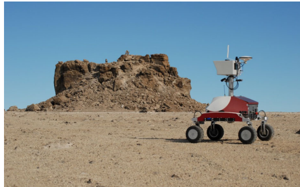
Fig. 1. NASA Ames K10 Red rover with the Optech ILRIS-3D Lidar operating at Haughton Crater.
