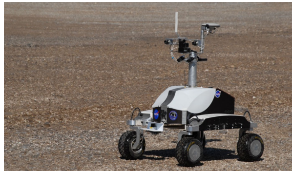
Fig. 2. NASA Ames K10 Black rover with the JPL CRUX ground-penetrating radar (GPR).
