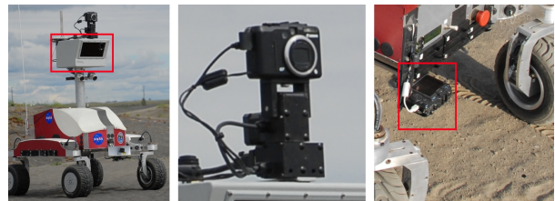
Figure 18. Recon instruments. Left to right: 3D scanning lidar (Optech ILLRIS-3D), panoramic imager (Canon G7 on pan/tilt), terrain imager (Canon G7).
