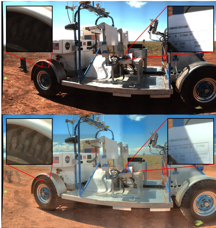
Figure 3. Inspection panoramas: top, LDR image; bottom, HDR image. The HDR image shows numerous features in deep shadow and bright highlight that are not visible in the LDR image.
