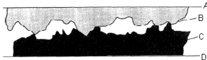
Figure 2.2. Microstructure of the resistive ink contact surface [13]
