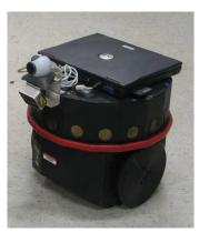
Fig. 1. Hardware environment in use for the 2004 edition of *Mobile Robot Programming Laboratory*: Nomad Scout with Dell laptop equipped with a PCMCIA wireless card and a Logitech USB webcam. The camera is fixed on the magnet support and facing forward. The circles on the side of the robot are its sonars.
