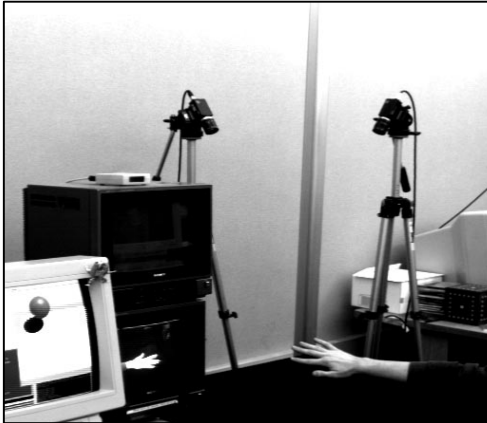
Figure 4.4: Experimental test bed for the DigitEyes system.
