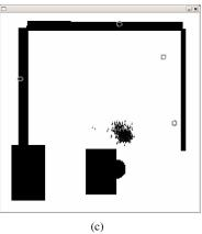
Figure 7: (a) The environment as seen by the stereo camera. (b) Particle filter localization using an *a priori* map before a landmark is observed. (c) The same particle filter estimate after a landmark is observed and an update occurs.
