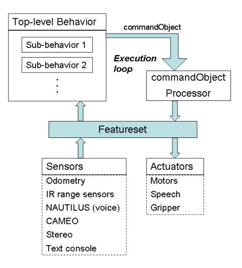
Figure 2: CMAssist Software Architecture
