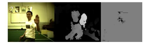
Figure 6: Stereo vision: color image from stereo image pair (left), calculated depth map (center), projected top-down occupancy map (right).
