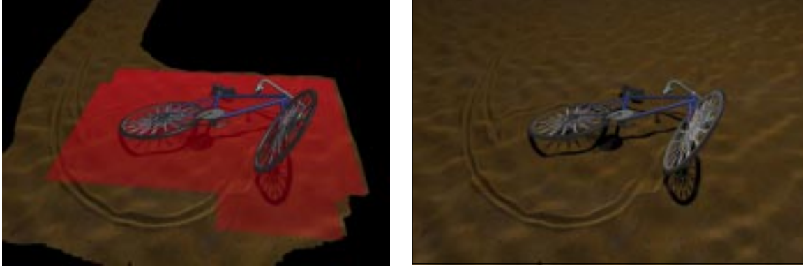
Figure 7: The left figure shows the ground area that has been created in the hash table. The currently active area is highlighted in red. The right figure shows the same scene rendered over the initial ground surface. There are approximately 37,000 columns in the active area and 90,000 stored in the hash table; the number of columns in the entire virtual grid is greater than 2 million.
