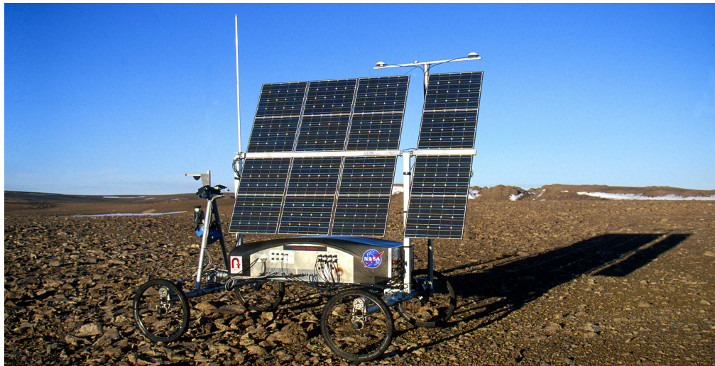
Figure 5-1: Hyperion Rover: Sun-synchronous navigation enabled solar powered travel over kilometers without the added complication and mass of a gimbal mechanism.
