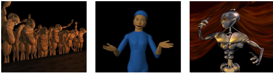
Simulated humanoid characters with different dynamics track human motion data to perform upper-body gesturing behaviors (Fig. 7).
