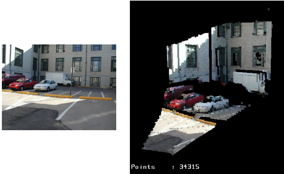
Figure 7: Example of a test scan-image observation with scan rendered with the image after calibration
