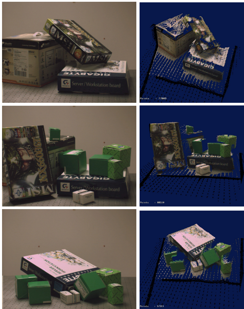
Figure 6: Examples of supplied test scan-image pairs with scans rendered with the image after calibration
