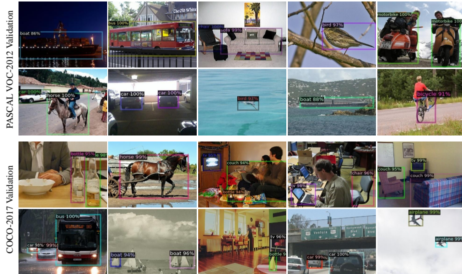
Fig. 1. Representative examples of 3-shot detection of AirDet on VOC-2012 validation and COCO validation dataset. Without fine-tuning, AirDet can robustly detect the novel unseen objects such as boat, bus, sofa, with merely three support images.
