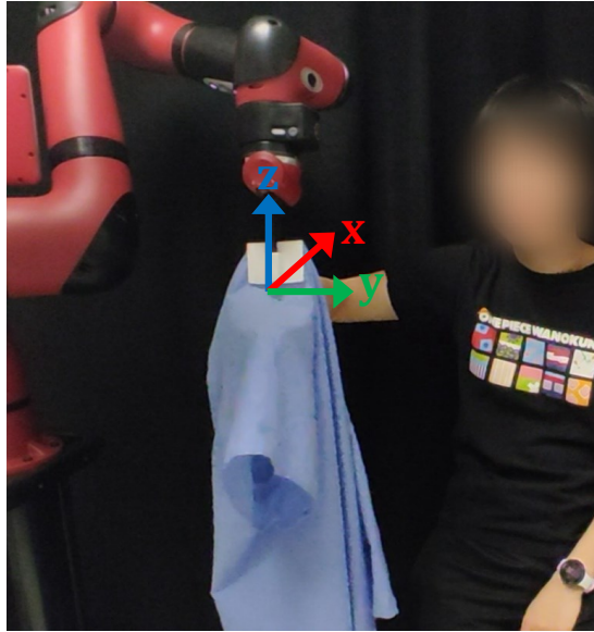
Figure A.1: Coordinate system in the real world.
