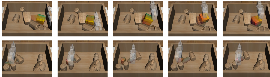
Figure A.9: Qualitative results for object pose alignment tasks in cluttered environments. HACMan shows complex non-prehensile behaviors that move objects to goal poses (shown as the transparent objects). The scene objects are colored in brown to distinguish from the target object to be manipulated to the goal pose.
