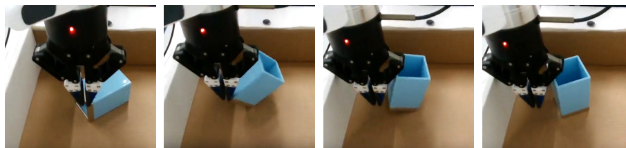
Figure A.16: An example of non-quasi-static motion. The figure shows an example of executing the motion parameters to flip a mug upright. After the gripper pushes against the edge of the mug (first two images), it relies on the inertia of the mug to finish the motion which is not quasi-static (last two images).
