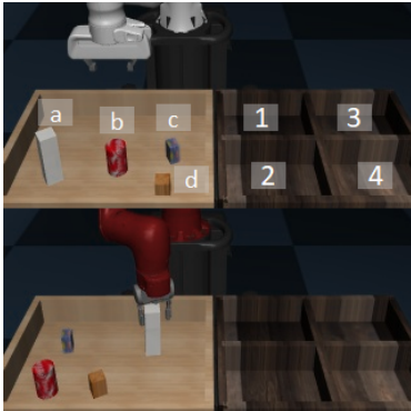
Figure 2.3: Our base environment is adopted from RoboTurk [145]. The 16 tasks consist of taking an object (a-b) to a bin (1-4). Top robot is agent and bottom is demonstrator.
