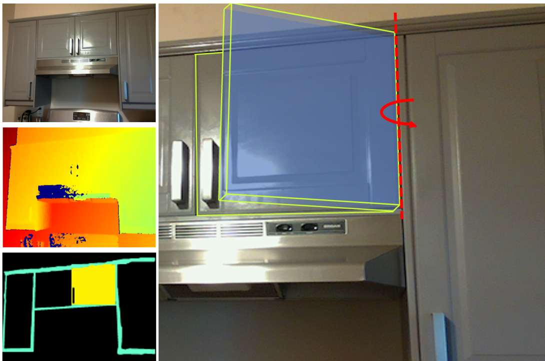
Figure 3.1: Predicting articulation mechanisms using FormNet. Given the inputs on the left (RGB-D image and segmentation masks of a pair of object parts), a neural network predicts the articulation type (revolute, prismatic, fixed, or unconnected) and appropriate articulation parameters (e.g., location and direction of revolute axis). The network is trained on synthetic data and infers articulation parameters via predicting motion residual flows.
