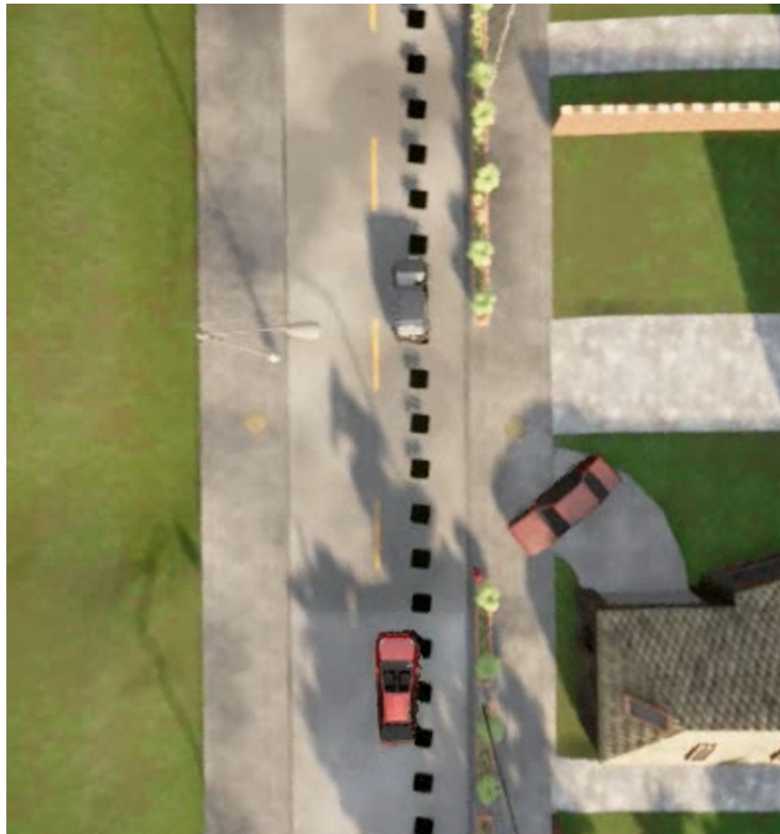
Figure 4.2: The overtake scenario in CARLA comprising an ego vehicle and a stationary vehicle parked in the path of the ego vehicle.
