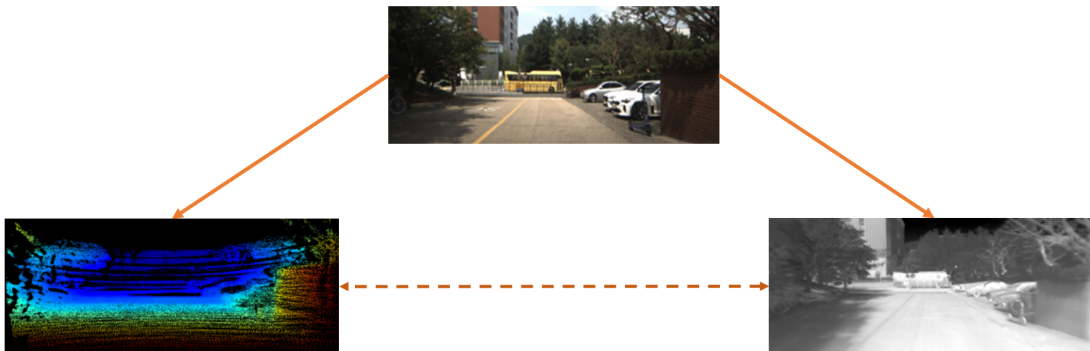
Figure 4.1: We show that binding LIDAR and thermal modalities to features to vision foundation models is effective to achieve zero-shot cross-modal place recognition.
