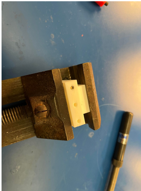
Figure 2.15: Remove the tang using the correctly sized tang break-off tool. Make sure that the tang does not stay inside the part
