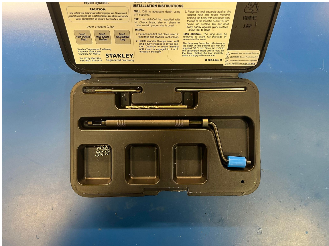
Figure 2.11: Parts required to correctly install Helicoils
