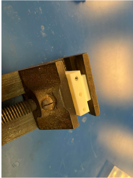
Figure 2.14: Make sure that the Helicoil is positioned one quarter-turn of the installation tool below the surface of the part
