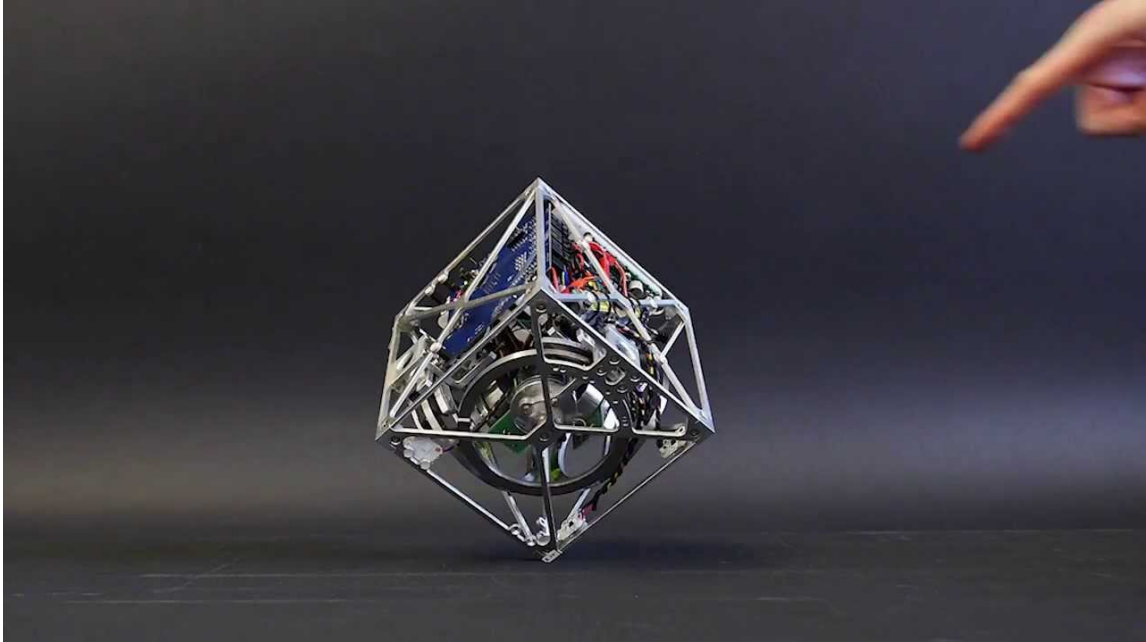
Figure 2.2: The Cubli, a RWA controlled robot [10]
