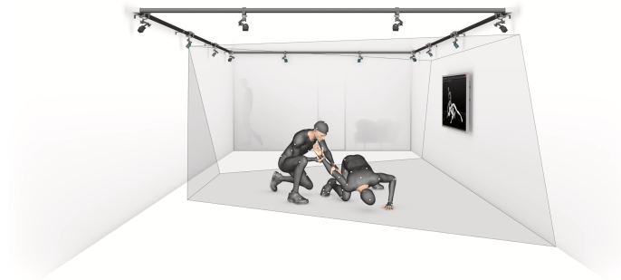
Figure 3.1: Motion capture setup for virtual production with two actors in a controlled and confined environment. The cameras are placed optimally on a height facing towards the actors such that they optimally cover the room with their view space. *Figure referenced from optitrack
