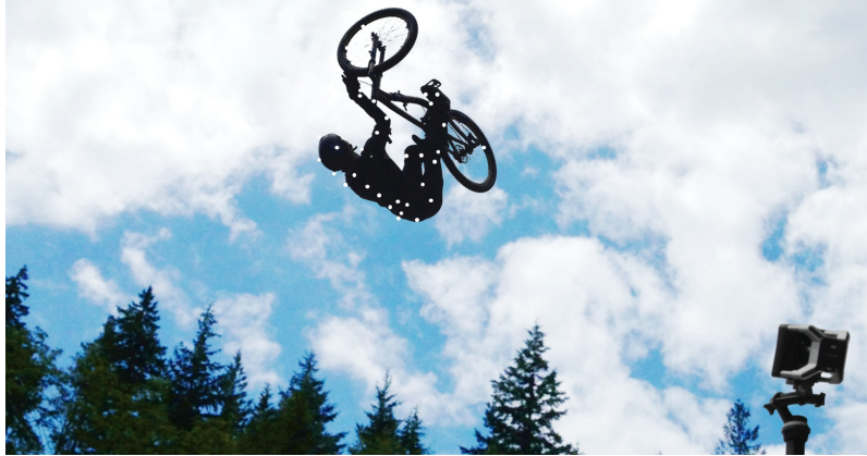
Figure 3.2: Ground motion capture setup in outdoor settings with no environmental occlusions using multiple tripod camera systems. *Figure referenced from optitrack
