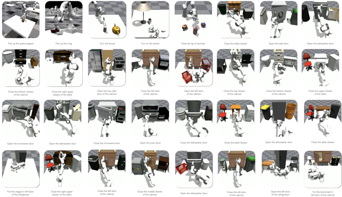
Figure 1.1: Gen2Sim is an automated generative pipeline of assets, tasks, task decompositions, and rewards functions for autonomous robotic skill learning in simulation. Here we show 32 generated tasks, concerning affordances of diverse types of object assets and their combinations.
