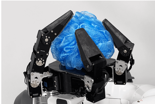
Figure 3.4: Data collection setup: Tactile data is collected by placing the object on the palm and executing a human-scripted interaction policy for motor babble.
