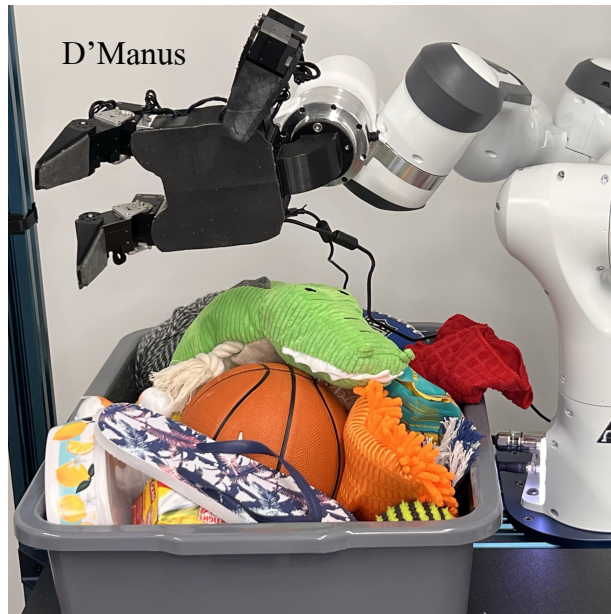
Figure 3.1: The D'Manus – a low-cost, 10 DoF, reliable prehensile hand with ReSkin [13] sensing.
