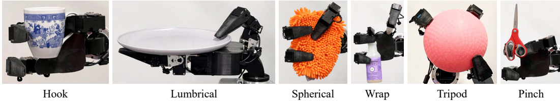
Figure 3.8: Illustration of the D'Manus grasping different objects with a variety of grasps [43, 156]
