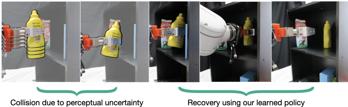
Figure 5.1: Due to uncertainty in the grasp of the object, the robot ends up making contact with the shelf during execution resulting in a collision as well as an in-hand slip failure. However, using the proposed recovery chaining framework, the robot recovers from the collision state and then hands over control to the nominal place skill. The learnt recovery also allows the robot to correct the slip by intentionally making contact with the shelf wall. Note that the policy is trained entirely in simulation.
