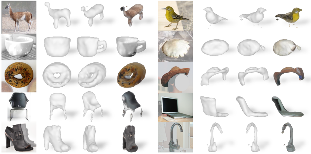
Figure 3.1: Given a single image, we predict a mesh with textures (rendered from the predicted view and a novel view). The models can learn directly from collections of images with only foreground masks, without supervision of mesh templates, multi-view association, camera poses, semantic annotations, etc. .
