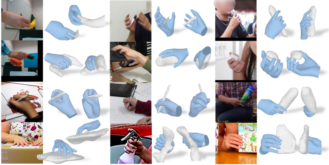
Figure 4.1: Given an RGB image depicting a hand holding an object, we infer the 3D shape of the hand-held object (rendered in the image frame and from a novel view).
