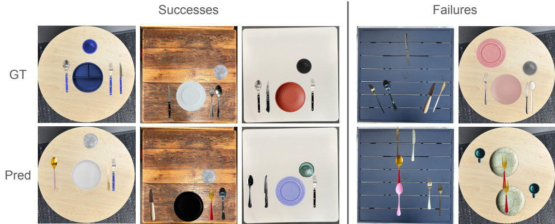
Figure 6.5: Qualitative results. On the top line we see ground truth images from our naturalistic preference data and on the bottom we see DegustaBot-LOGMA’s predictions, lifted into the image domain. On the left side of the image we see three examples where DegustaBot-LOGMA predicts similar arrangements to the ground truth image. On the right we see some failure cases.
