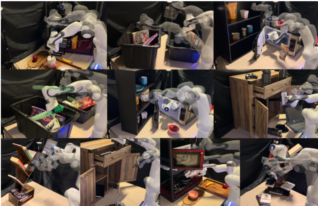
Figure 10.1: Neural Motion Planning at Scale in the Real World. We train a single neural network policy to solve motion planning problems across diverse tabletop setups enabling it to generate collision free motions for entirely unseen tasks such as placing books in bookcases, transferring items from shelves to microwaves, rearranging electronics from a drawer into a cabinet and moving irregular items between bins.
