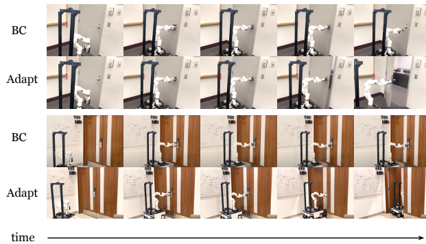
Figure 8.7: Online Improvement Visualization: In the third row, the pretrained BC policy completely fails to open the “push” door. With continual practice, the robot is able to achieve a high success rate after online adaptation in the fourth row. For doors with knobs, in the first row, using the vanilla grasp does not establish a robust grasp pose, our adaptation method enables the robot to adjust the grasp pose through online adaptation.
