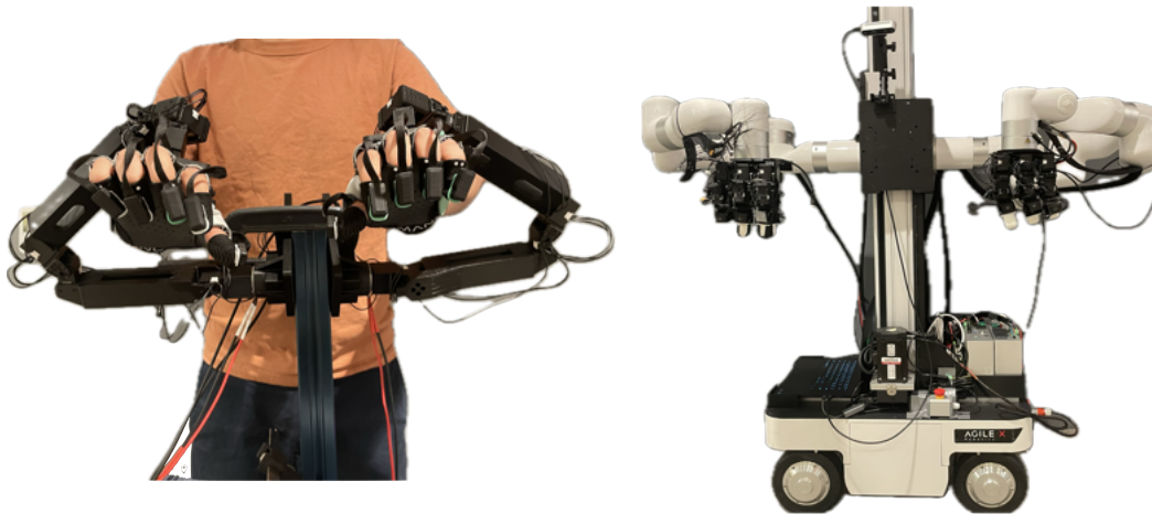
Figure 9.2: Mobile bimanual teleoperation system. Left: An operator strapped into BiDex. Right: Our bimanual robot setup including two xArm robot arms, two LEAP Hands [362] and three cameras on an AgileX base.
