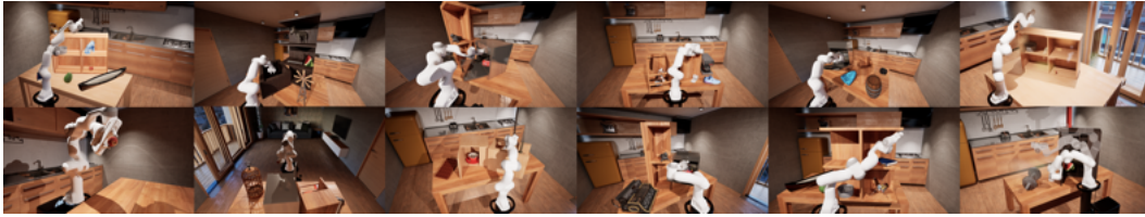
Figure 10.2: Visualization of Diverse Simulation Training Environments: We train Neural MP on a wide array of motion planning problems generated in simulation, with significant pose, procedural asset, and mesh configuration randomization to enable generalization.
