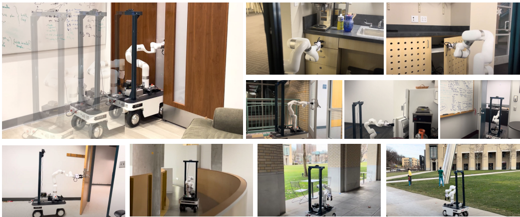
Figure 8.1: Open-World Mobile Manipulation System : We use a full-stack approach to handle articulated objects such as real-world doors, cabinets, drawers, and refrigerators in open-ended unstructured environments.
