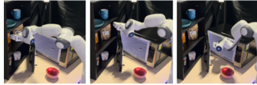
(a) Sampling-based planners struggle with tight spaces, a regime in which Neural MP performs well.
