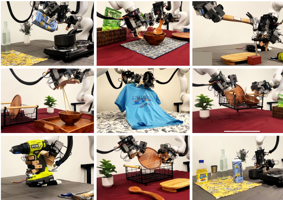
Figure 9.1: Bimanual Dexterity: Our teleoperation data collection system can perform various complex tasks including pouring, hammering, chopstick picking, hanger picking, picking up basket, drilling, plate pickup and pot picking, using a bimanual dexterous system.
