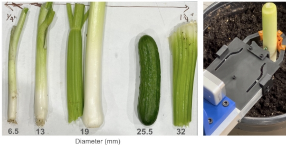
Figure 7.4: Gripper Insertion Testing: (a) Vegetable products of varying diameter (b) Gripper insertion testing using leek
