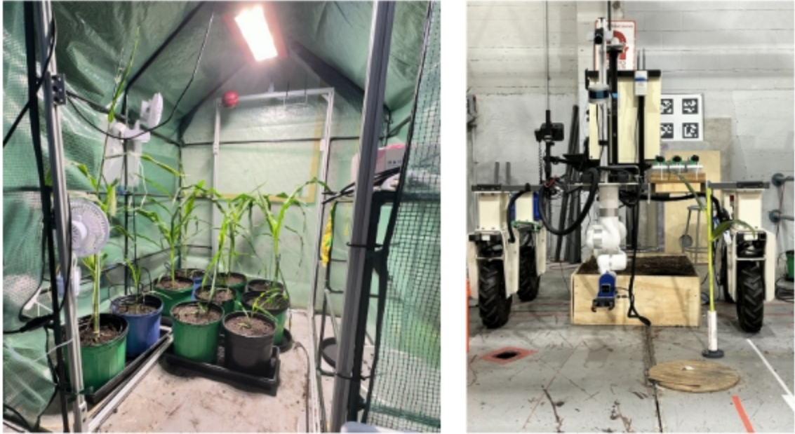
Figure 7.5: Testing with corn: (a) Growing cornstalks in an indoor greenhouse (b) Testing perception insertion motion sequence with a mock cornstalk
