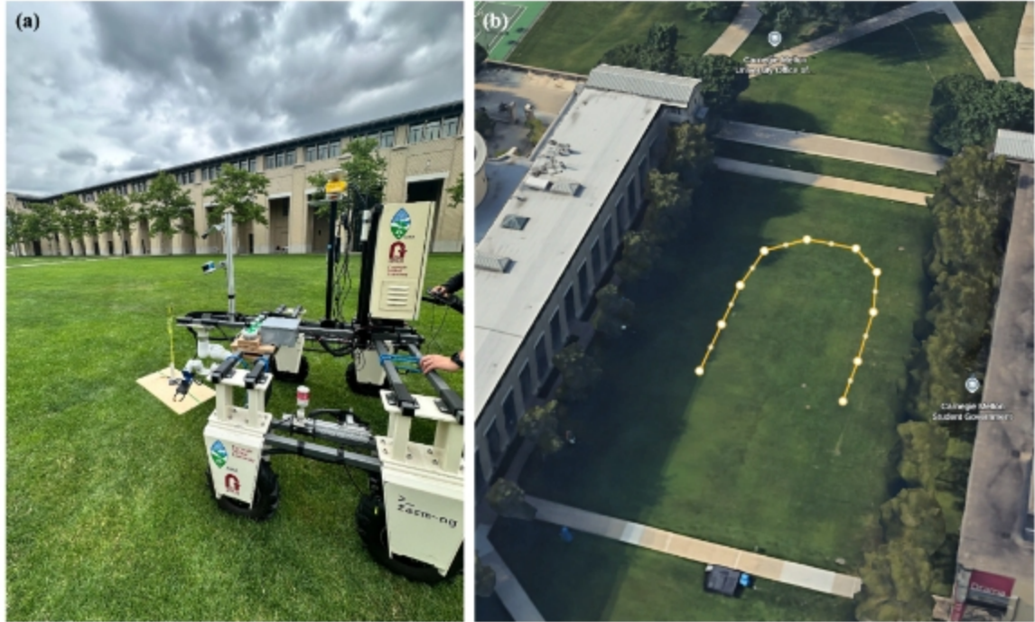
Figure 7.9: (a) Navigation Integration testing on campus quad (b) Planned path based on the waypoints
