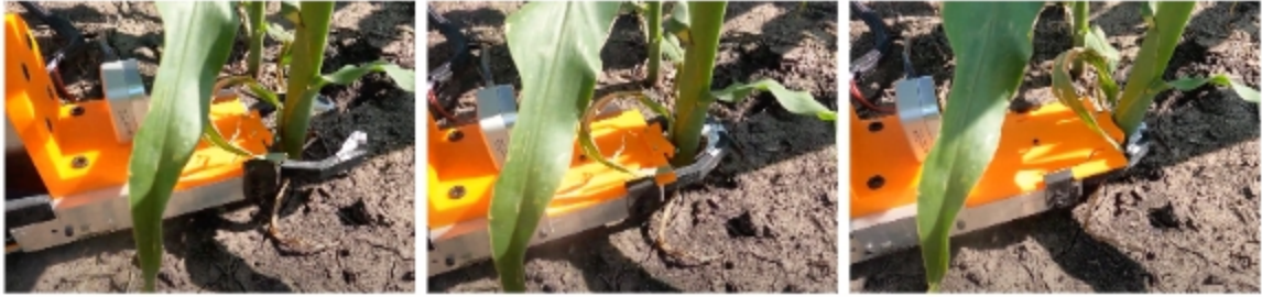
Figure 4.3: Gripper motion for grasping the stalk and inserting sensor.
