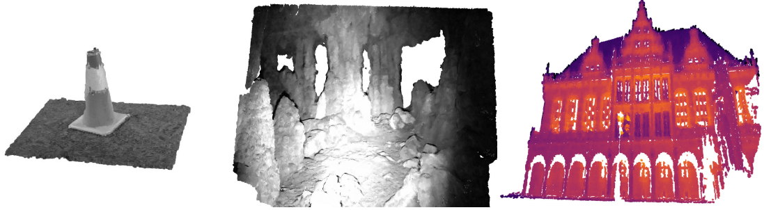
Figure 1.2: The methodology proposed in Chapter 6 enables multi-modal reconstruction at varying scales. Without modifying the model complexity parameters, the methodology models depth and grayscale data of small objects ( 1\text{ m} \times 1\text{ m} safety cone in the left image) and complex environments ( 10\text{ m} \times 5\text{ m} cave in the center image) while also modeling depth and thermal data of (right) large-scale buildings ( 42\text{ m} \times 28\text{ m} ) [18]. A supplementary video may be found at https://youtu.be/TCn5KB1m5P0 .
