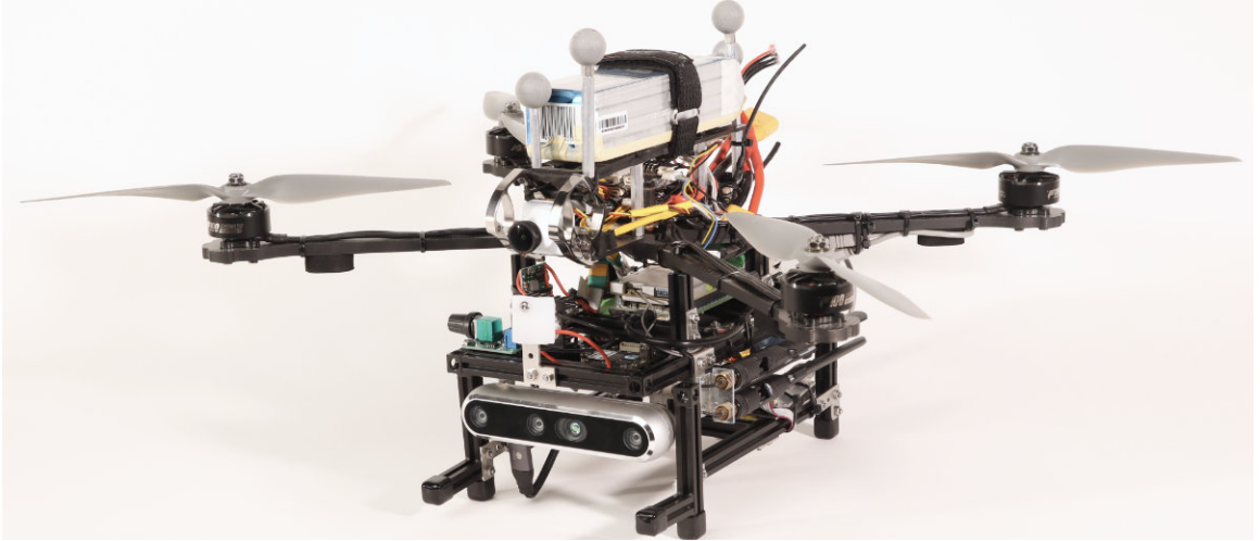
Figure 5.3: The robot used in the field experiments is equipped with a forward-facing Intel Realsense D455, downward-facing mvBluefox global shutter color camera, and Pixracer flight controller.
