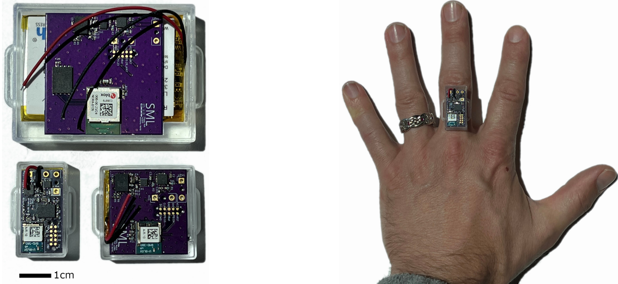
(a) Sensors assembled and in their enclosures
