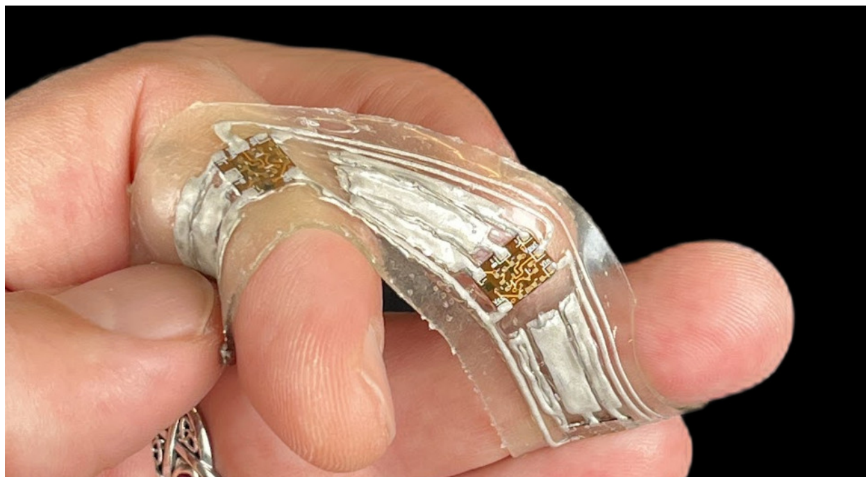
Figure 4.1: A stretchable strain gauge built using a simple notch filter.
