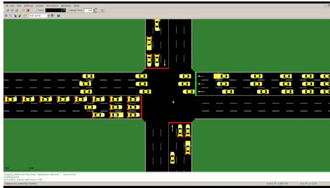
Figure 15: Example of road network simulation by SUMO
